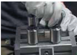
1. Position the SXA001 hose splitter in a bench vice and grip firmly. Spread the rollers apart.
