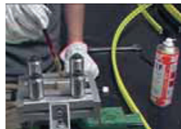
2. Lubricate the top of the cutting blade with grease.
