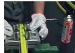
4. Firmly support the hose keeping it parallel with the reference lines and held in position by the rollers.
