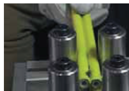
6. Hold the hose and pull slowly being careful to keep the hose in a horizontal position.
