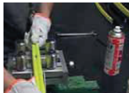
3. Hold the hose with both hands and push downwards until the blade has completely penetrated between the hoses.
